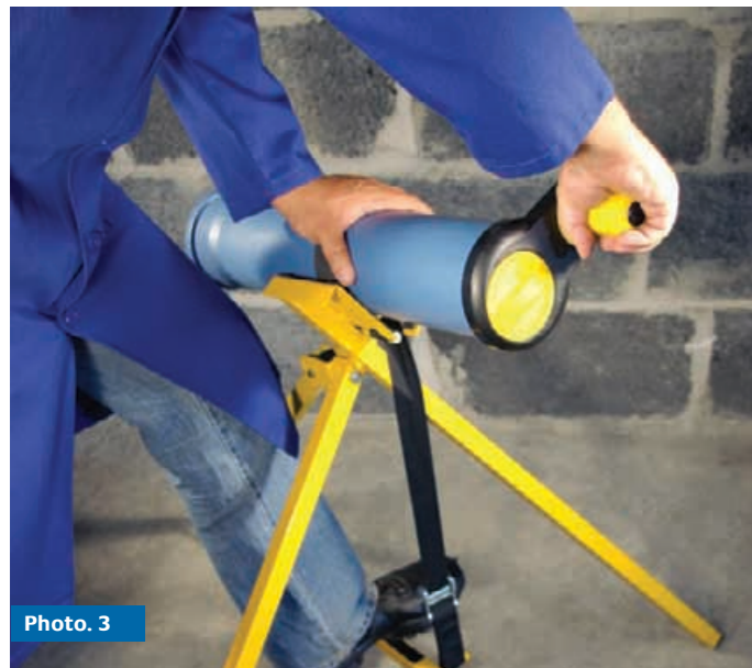
Another important factor prior to making the connections is to bevel the pipe end properly, using a chamfering tool or coarse file to provide a 15° bevel on the end of the pipe.
