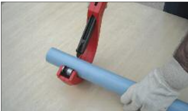
2. Cut pipe to required length.
