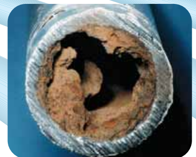
Durapipe superFLO resists the limescale build-up common in most metal pipe materials as shown in the picture above.
