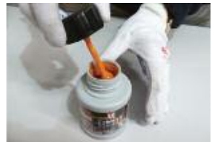
6. Stir welding polymer.
